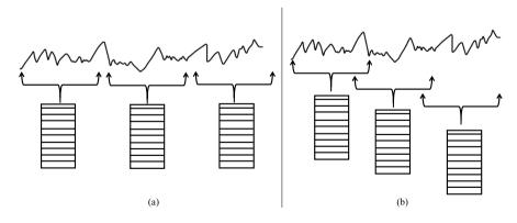
Fig. 3. Sliding window illustration (a) Windowing without overlap (b) Windowing with overlap.
